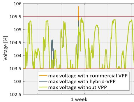
Figure 3: Market driven use case – Grid simulations show the possible benefits (from grid perspective) of a hybrid-VPP compared to a pure commercial VPP.
