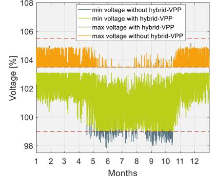
Figure 5: Grid driven use case – Grid simulations show that necessary grid reinforcements can be postponed by using a hybrid-VPP.
